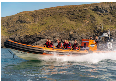
RIB: a ridged inflatable boat, solid hull and inflatable tubes on the sides
